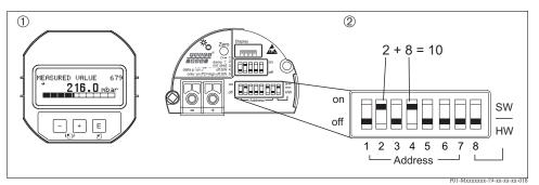
Fig. 6: Setting the device address via DIP switches
