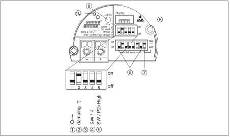
Fig. 5: PROFIBUS PA electronic insert
