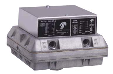
Model RHLGP-A High-Low Gas Switch Recycle Type The Model A is a high-low gas pressure switch that monitors pressure and cuts off the electrical control circuit when pressure drops below or rises above the desired setpoint. The high and low gas pressure settings are adjustable. All models are available in reset or recycle type.
