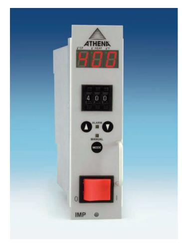
Athena's Series IMP Modular Hot Runner controller is a microprocessor-based, single-zone temperature controller specifically designed for runnerless molding applications. The controller is fully self-tuning, with built-in diagnostics, and features an easy-to-use operator keypad with simultaneous process and set point displays and discrete indicators for heat output, alarm, degrees F/C, manual/closed loop mode, and CompuStep<sup>®</sup>.
