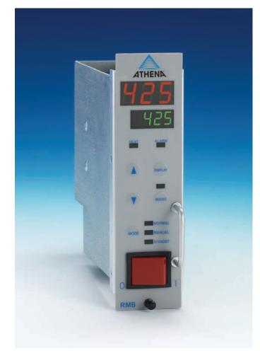
Athena's Series RMB Modular Hot Runner controller is a microprocessor-based, single-zone temperature controller specifically designed for runnerless molding applications. The controller is fully self-tuning, with built-in diagnostics, and features an easy-to-use operator keypad with simultaneous process and set point displays and discrete indicators for heat output, alarm, degrees F/C, manual/closed loop mode, and CompuStep<sup>®</sup>.
