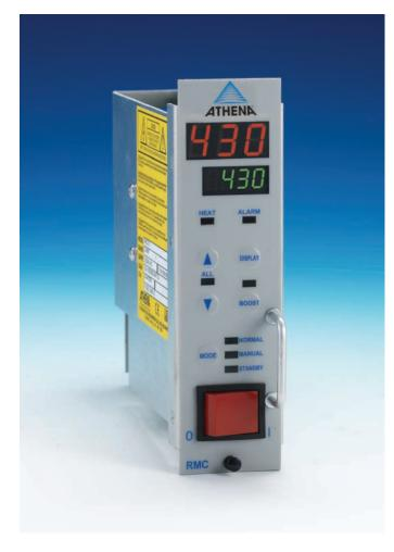
Athena's Series RMC Modular Hot Runner controller is a microprocessor-based, single-zone temperature controller specifically designed for runnerless molding applications. The controller is fully self-tuning, with built-in diagnostics, and features an easy-to-use operator keypad with simultaneous process and set point displays and discrete indicators for heat output, alarm, degrees F/C, manual/closed loop mode, and CompuStep<sup>®</sup>.
