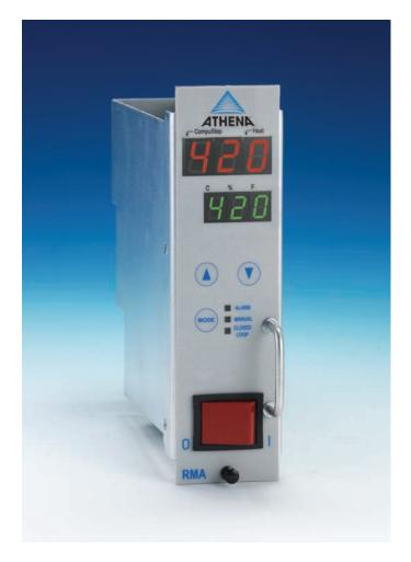
Athena's Series RMA Modular Hot Runner controller is a microprocessor-based, single-zone temperature controller specifically designed for runnerless molding applications. The controller is fully self-tuning, with built-in diagnostics, and features an easy-to-use operator keypad with simultaneous process and set point displays and discrete indicators for heat output, alarm, degrees F/C, manual/closed loop mode, and CompuStep<sup>®</sup>.
