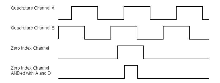
Our quadrature signal conditioner board can be used for quadrature position (with Basic or Extended main board) or for quadrature rate (with Extended main board). Two quadrature signals, which are 90° out of phase, are applied to the Channel A and B inputs. Their phase relationship determines whether the count is up (+) or down (-). A zero index signal may be applied to Channel Z as a position reference.
