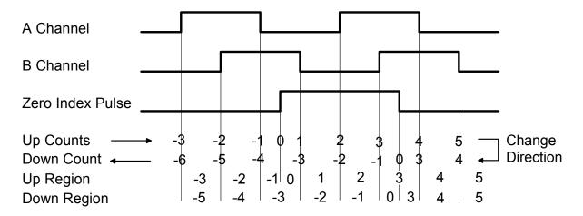
It follows that a wide zero index signal causes a discrepancy in the count in the regions between transitions when counting up and counting down. To correct this situation, AND the zero index signal with the A & B channel signals. Assume for this example the zero index is ANDed with the inverse of A (/A) and the inverse of B (/B) to produce ZIY as shown below.
