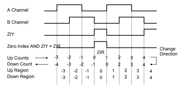
By ANDing the zero index signal with the A & B channels, there is no regional discrepancy between counting up and counting down.
