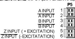
Z input or excitation is jumper selectable. With differential quadrature inputs and an external power supply, connect ground of the external supply to Pin 6 of P1.
