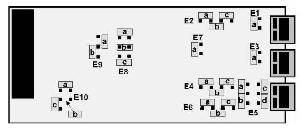
Note: Letters indicate jumper position. Jumpers are installed on pins adjacent to letters.
