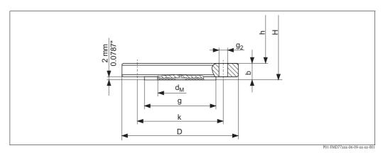
Process connection FMD77, high-pressure side, JIS flange, material AISI 316L (1.4435)
