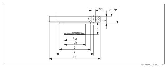
Process connection FMD77, high-pressure side EN/DIN, material AISI 316L
