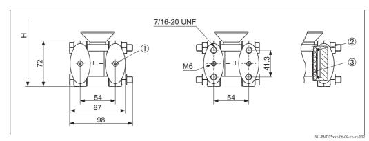
Left: Process connection PMD75, version W, prepared for diaphragm seal mount Right: Position of the copper ring seal (Nuts are always located on the minus side)
