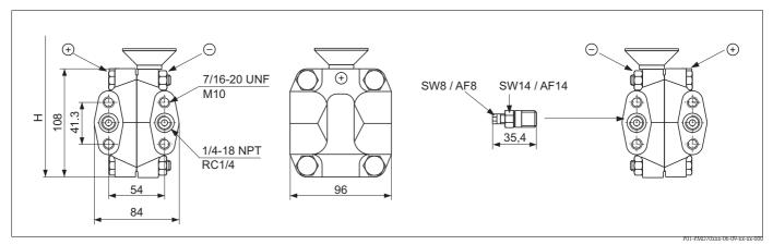
Process connection PMD70, oval flange (Nuts are always located on the minus side)
