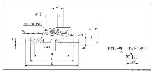
Process connection FMD76, high-pressure side: EN/DIN flange, Low-pressure side: connection 1/4-18 NPT Application limits for version "G" in feature 70 "Process connection low-pressure side" with PVDF Inlay: MWP 10 bar (150 psi), OPL max. 15 bar (225 psi), process temperature limits T = -10 to +60°C (+14 to +140°F)
