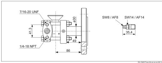
Low-pressure side: connection 1/4-18 NPT, mounting optionally 7/16-20 UNF incl. 1 vent valve AISI 316L (1.4404), Side flange material of the basic device: AISI 316L (1.4435 or 1.4404) High-pressure side, see the following section "Process connections, high-pressure side FMD77" Nuts are always located on the plus side)
