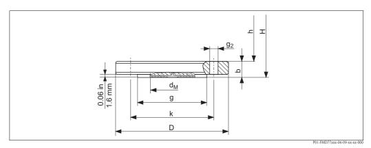
Process connection FMD77, high-pressure side ANSI flange, material AISI 316/316L
