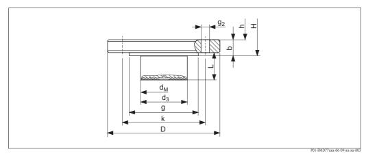
Process connection FMD77, high-pressure side ANSI flange, material AISI 316/316L
