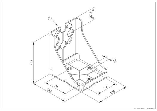
Mounting bracket for wall and pipe-mounting Materials: Screws and washers A2-70 or A4, bracket and retainer 1.4301.
