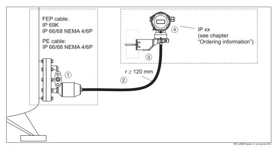
In the case of the "separate housing" version, the sensor is delivered with the process connection and cable ready mounted. The housing and a mounting bracket are enclosed as separate units. The cable is provided with a socket at both ends. These sockets are simply connected to the housing and the sensor.
