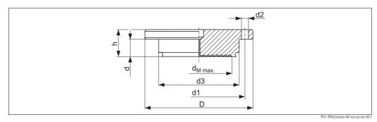
Process connection PMP55, material AISI 316L, surface roughness of the surfaces in contact with the medium  $Ra \le 0.76 \ \mu m$  (29.9  $\mu in$ ) as standard. Lower surface roughness on request.
