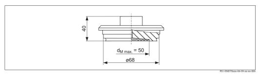
Process connection FMD78, Material AISI 316L, surface roughness of the surfaces in contact with the media  $R_a \leq 0.76$   $\mu m$  (29.9  $\mu$ in) as standard. Lower surface roughness on request.
