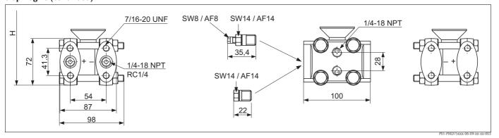
H Device height see ightarrow ightharpoonup 41, "Device height H" section (Nuts are always located on the minus side)
