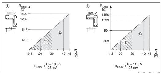
Load diagram, observe the position of the jumper and the explosion protection ( $\rightarrow \triangle$  20, "Measuring a 4 to 20 mA test signal" section.)
