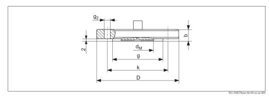
Process connection FMD78, EN/DIN or JIS flange, material AISI 316L
