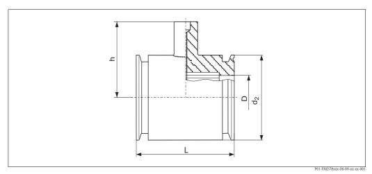
Process connection FMD78, material AISI 316L, surface roughness of the surfaces in contact with the media  $R_a \le 0.8 \, \mu m \, (31.5 \, \mu in)$  as standard. Lower surface roughness on request.
