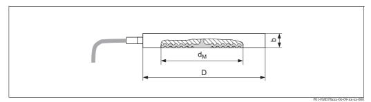
Process connection FMD78, material AISI 316L
