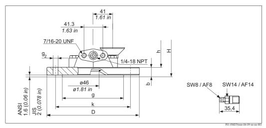
Process connection FMD76, high-pressure side: ANSI or JIS flange, Low-pressure side: connection 1/4-18 NPT
