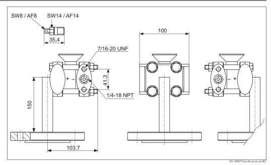
Low-pressure side: connection 1/4-18 NPT, mounting optionally 7/16-20 UNF incl. 1 vent valve AISI 316L (1.4404), Side flange material of the basic device: AISI 316L (1.4435 or 1.4404) High-pressure side, see the following section "Process connections, high-pressure side FMD77" (Nuts are always located on the minus side)
