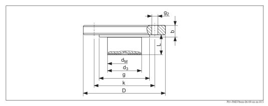
${\it Process connection FMD78, ANSI flange, material AISI~316/AISI~316L}$
