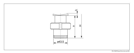
Universal adapter incl. silicone molded seal
