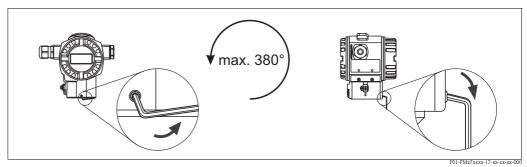
Aligning the housing by releasing the setscrew T14 and T15 housing: 2 mm (0.08 in) Allen screw; T17 housing: 3 mm (0.12 in) Allen screw
