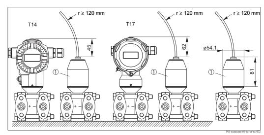
Reduction of the installation height of the process connection when using the separate housing.
