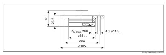
Process connection FMD78, surface roughness of the surfaces in contact with the media  $R_a \le 0.76 \, \mu m$  (29.9  $\mu$ in) as standard. Lower surface roughness on request.
