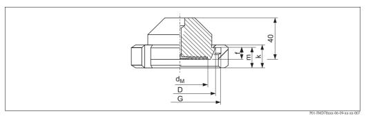
Process connection FMD78, material AISI 316L, surface roughness of the surfaces in contact with the media  $R_a \le 0.76~\mu m~(29.9~\mu in)$  as standard. Lower surface roughness on request.
