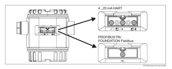
The operating keys located externally on the device work on the Hall sensor principle. As a result, no additional openings are required in the device. This guarantees:
