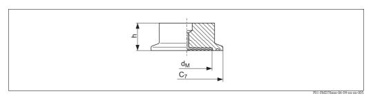
Process connection FMD78, material AISI 316L, surface roughness of the surfaces in contact with the media  $R_a \leq 0.76 \, \mu m$  (29.9  $\mu$ in) as standard. Lower surface roughness on request.
