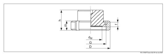
Prozessanschluss FMD78, material AISI 316L, surface roughness of the surfaces in contact with the medium Ra  $\leq$  0.76  $\mu m$ (29.9 µin) as standard. Lower surface roughness on request.
