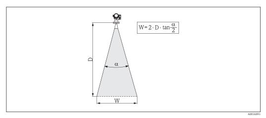
■ 12 Relationship between beam angle a, distance D and beamwidth diameter W
