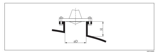
• 14 Nozzle height and diameter for horn antenna with slip-on flange
