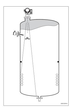
Avoid any installations (point level switches, temperature sensors, braces, vacuum rings, heating coils, baffles etc.) inside the signal beam. Take into account the beam angle  $( \rightarrow \square 37)$ .
