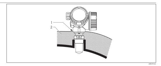
If process temperatures are high, the device must be included in normal tank insulation to prevent the electronics heating up as a result of heat radiation or convection. The insulation may not exceed beyond the neck of the housing.
