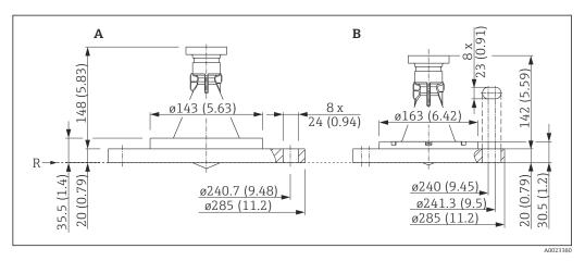
E 26 FMR50 with slip-on flange 6"/DN150; dimensions: mm (in)
