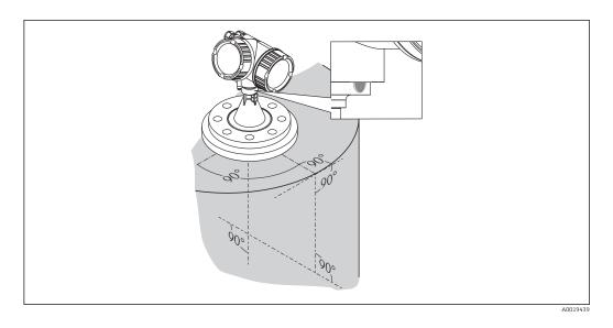
P Depending on the device version the marking may be a circle or two short parallel lines.
