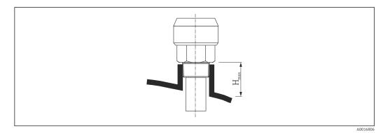
$\blacksquare$  13 Nozzle height for horn antenna, encapsulated (FMR50);  $H_{max} = 60 \text{ mm} (2.36 \text{ in})$
