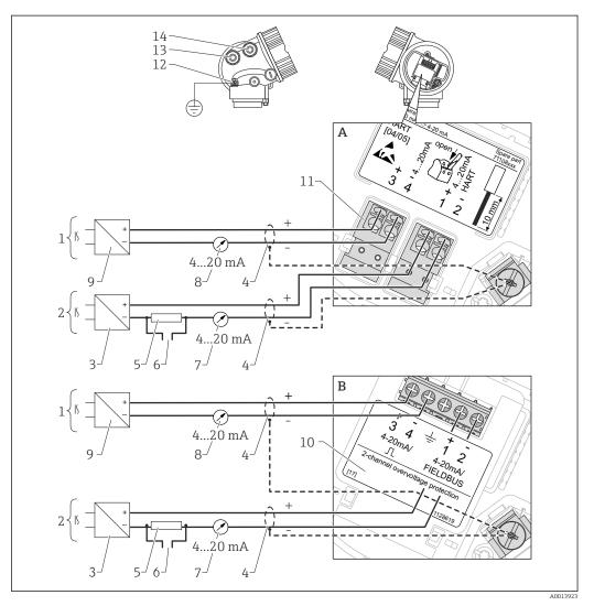
E 4 Terminal assignment 2-wire, 4-20 mA HART, 4...20mA
