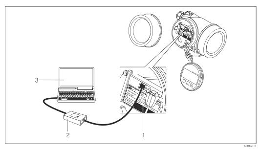
Service interface (CDI) of the measuring device (= Endress+Hauser Common Data Interface) Commubox FXA291
