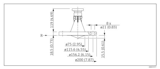
24 FMR50 with slip-on flange 3"/DN80; dimensions: mm (in)
