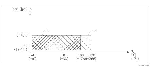
■ 18 FMR50: Admissible range of process temperature and process pressure
