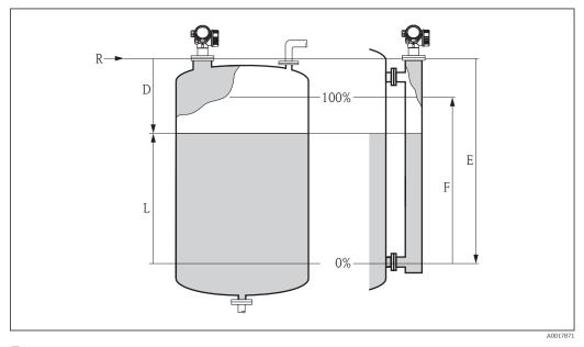
I Setup parameters of the Micropilot
