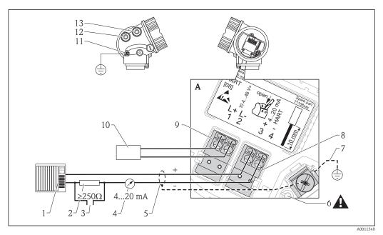
☑ 5 Terminal assignment 4-wire; 4-20mA HART (10.4 to 48 VDC)
