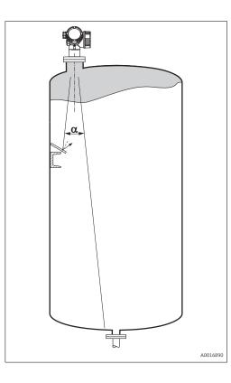
Metallic screens mounted at a slope spread the radar signal and can, therefore, reduce interference echoes.
