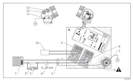
Image: Terminal assignment 4-wire; 4-20mA HART (90 to 253 VAC)
