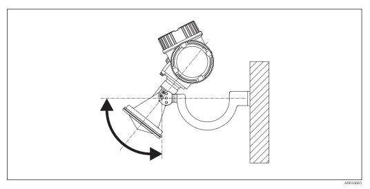
🖻 15 Installation of the horn antenna with mounting bracket
