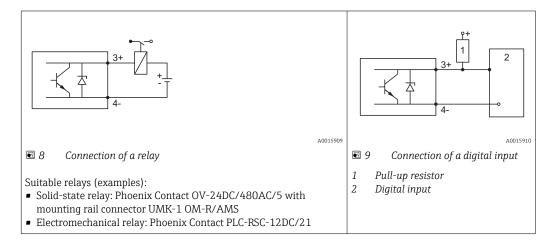
For optimum interference immunity we recommend to connect an external resistor (internal resistance of the relay or Pull-up resistor) of <  $1000 \Omega$ .
