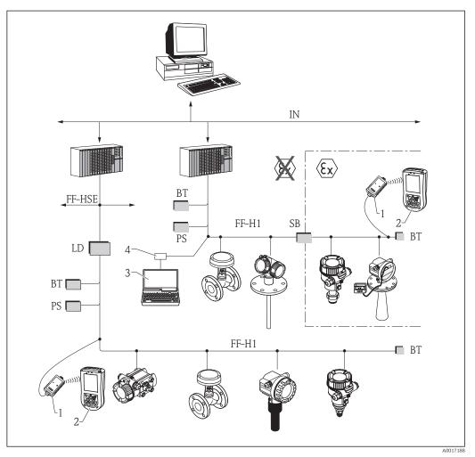
FOUNDATION Fieldbus system architecture with associated components
