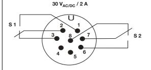
\*Control 1<->GND: Start-Dosing Control 2<->GND: Stop-Dosing
