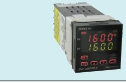
**The 16L Series Temperature/Process FM Approved Limit Controls** set a new standard in 1/16 DIN limit controls. The 16L offers universal input (10 thermocouple types, 4 RTD types, voltage, and current), single set point or dual set point. Standard features include remote reset capability, peak/valley indication, open sensor protection, input rate of change protection, and much more.
