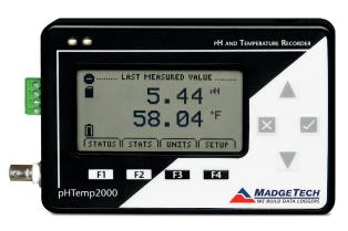
directly connecting an RTD to the pHTemp2000. Temperature compensation is automatically done internally to the unit.
