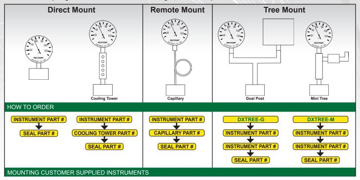
REOTEMP can mount and fill other manufacturers' instruments and diaphragm seals. Use the following part number designators and contact the factory for pricing.
