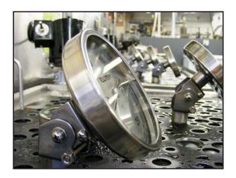
REOTEMP uses a combination of fixed point calibration cells and fluid-filled calibration equipment to perform calibrations from -196°C to 600°C (-320°F to 1112°F). We provide calibration for metrology and industrial customers in nearly every process market. Our friendly and knowledgeable technicians will ensure your sensors have the accuracy required for your application.
