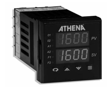
The Athena 16C is a 1/16 DIN panel mounted, autotuning controller that can be used for precise control of a single loop with two independent outputs fieldconfigurable as direct acting, reverse acting or alarm. RS-232 or RS-485 communications interfaces are available, and two digital LED displays provide visual indication of various controller functions.
