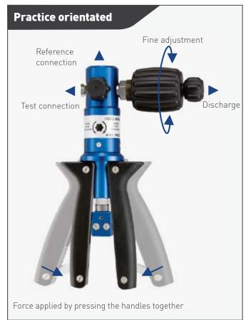
The required test pressure is initially generated using the handles and then adjusted precisely with the fine adjustment valve. As a result, the pressure on both instruments is the same.
