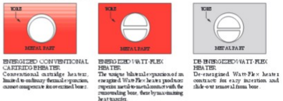
Figure 1: Watt-Flex Expansion Comparison
