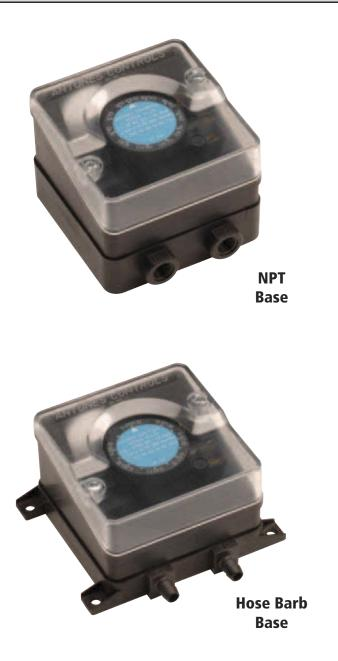
The Versa Plus Air is a highly accurate air pressure switch that monitors positive, vacuum, or differential air pressure. The integrated contacts make or break circuits to a desired setpoint. The omega spring design provides repeatability and accuracy. It is compact, easy to install, and available in various mounting configurations.
