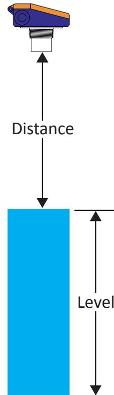
**1 = Level:** subtracts the measured target distance from the user defined Empty Distance to provide a depth of level measurement. Required parameter settings: Units, Full Distance, Empty Distance.
