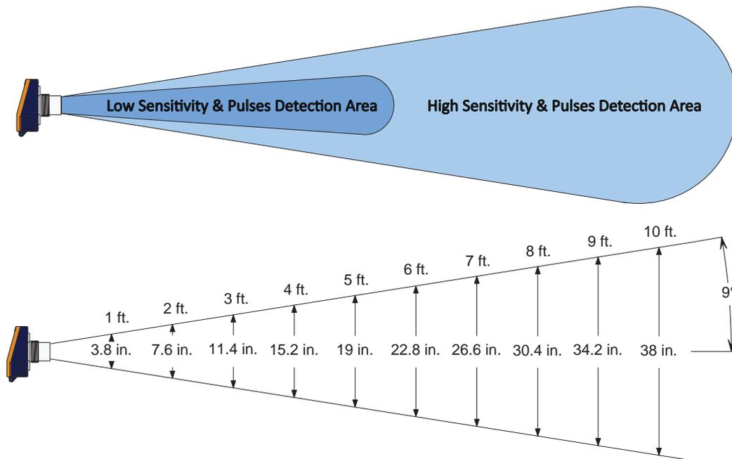
Typical beam spread of an ultrasonic sensor operating at maximum sensitivity setting.
