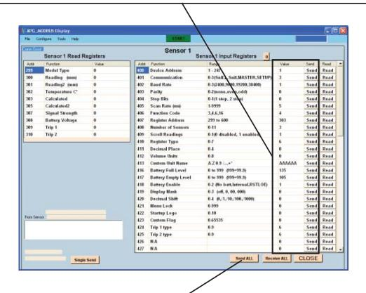
**Step 11:** To change multiple parameters, individually click on the values you wish to change, enter the desired values, then click the "Send All" button at the bottom of the window to write all the values to the MND.
