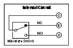
Switch rating (resistive) 250 V 10 A AC
