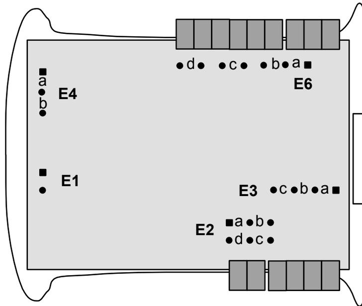
\* The termination resistor jumper settings should only be selected if the transmitter is the last device on an RS485 line longer than 200 feet (60 m).
