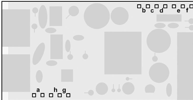
1. Letters indicate jumper position. Jumpers are installed on pins adjacent to letters.
