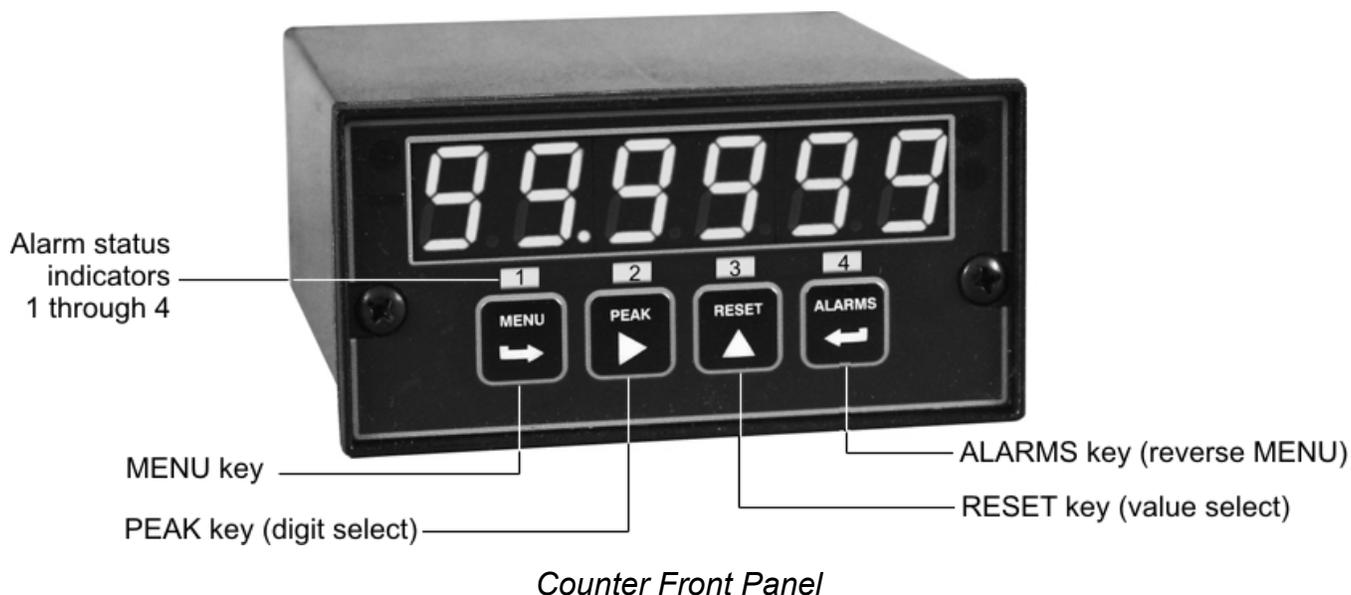
There are four front panel keys, which change function for the **Run Mode** and **Menu Mode**, effectively becoming eight keys. The keys are labeled with alphanumeric captions (MENU, PEAK, RESET, ALARMS) for the Run Mode and with symbols (➡ right arrow, ▶ right triangle, ▲ up triangle, ← left arrow) for the Menu Mode.
