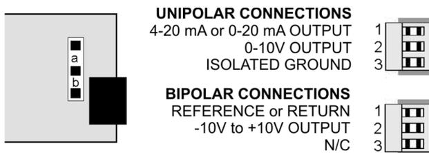
Unipolar current or voltage: Jumper **a**
