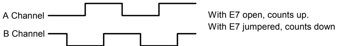
The board has jumpers that allow counting by 1, 2 or 4 counts per cycle of the A or B signals. The edges that are counted are:
