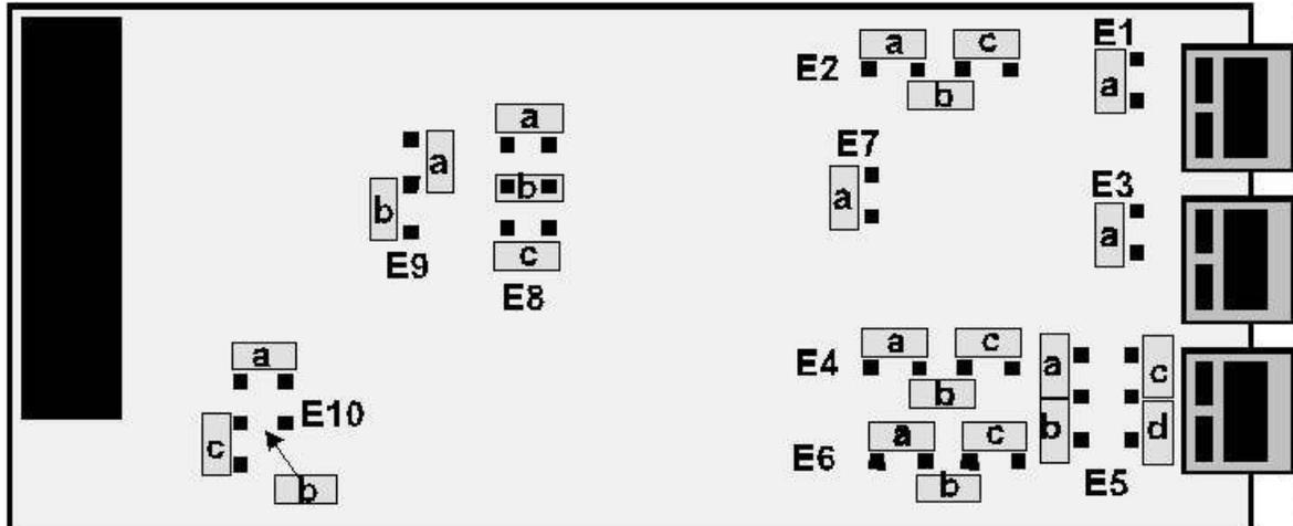
Note: Letters indicate jumper position. Jumpers are installed on pins adjacent to letters.
