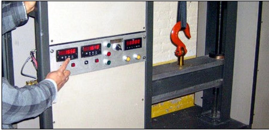
Seat belt tensile strength testing using Y800 Plus digital panel meters. The three meters display Force, Displacement and Speed.
