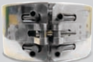
5/16 diameter stainless steel coolant tubes for long life.
