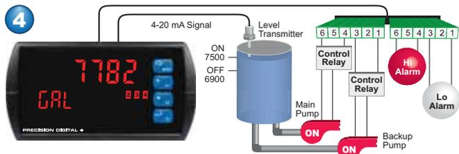
Relay #2 trips the High Level Alarm at 7500 gallons and resets at 6900 gallons.
