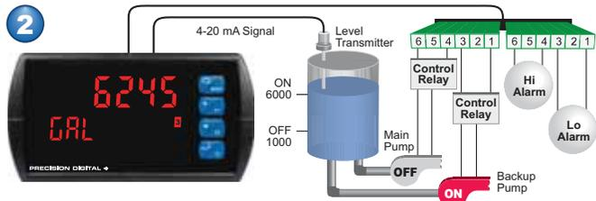
With the Pump Alternation feature activated, the next time the level reaches 6000 gallons, relay #3 transfers and starts the backup pump.
