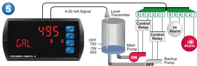
Relay #1 trips the Low Level Alarm at 495 gallons and resets at 750 gallons.
