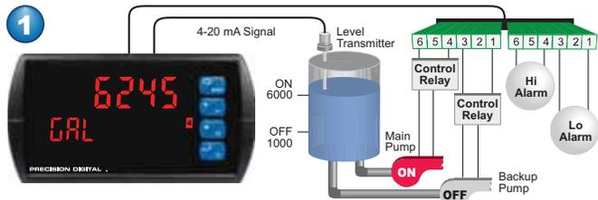
Relay #4 turns the main pump on at 6000 gallons and turns it off at 1000 gallons.
