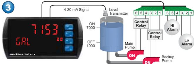
If the backup pump is not able to keep up, and the level reaches 7000 gallons, relay #4 transfers and starts the main pump as well.
