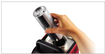
The optimum thermal coupling from the block to test item is achieved with the correct adapter sleeve. With the aid of the adapter sleeve, straight temperature sensors of virtually any length and diameter can be calibrated. The dry block covers the entire temperature range without the need to change the calibration medium. Viscosity, flash points or outgassing are of no concern.
