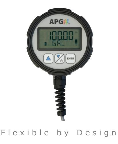
The MND Modbus Network Display provides a local display that can be wired to a local Tank Cloud network, or modbus sensor, displaying readings from any of the sensors in the network (up to ten). It is easy to use and very flexible. The MND can operate in either a master or sniffer mode. With the ability to listen in on sensors or poll sensors for current readings, the MND provides a valuable display option for your network.
