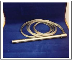
To install - mount heater through oven wall, cut cable entry holes in box, wire 120 VAC power to terminal strip heater connection and you're done. Low watt density, long life heater glows continuously (no controls) \*\*\*Optional 5/8" x 1/2" NPT compression fitting available for easy heater mounting.
