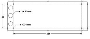
Figure 1 - Mounting the indicator in the panel cut-out.
