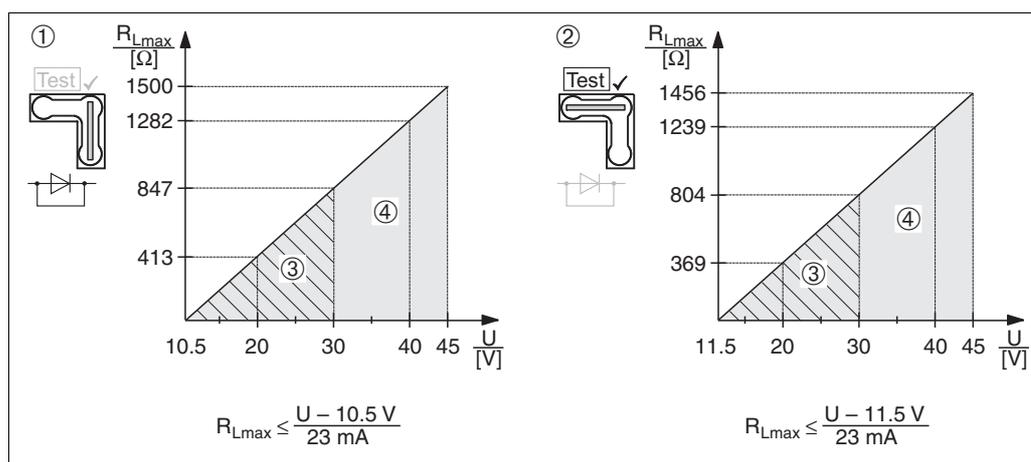
Load diagram, observe the position of the jumper and the explosion protection (→ 20, "Measuring a 4 to 20 mA test signal" section.)
