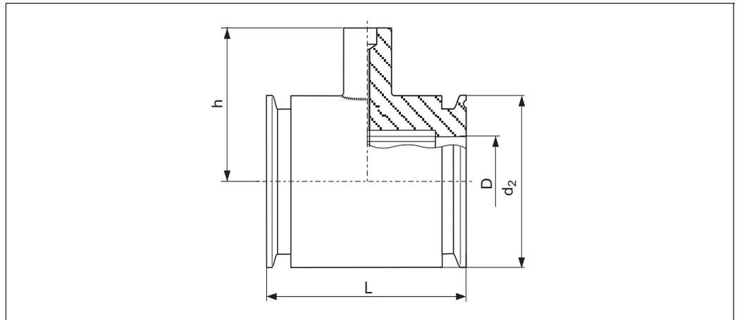
Process connection FMD78, material AISI 316L, surface roughness of the surfaces in contact with the media  $R_a \leq 0.8 \mu\text{m}$  (31.5  $\mu\text{in}$ ) as standard. Lower surface roughness on request.
