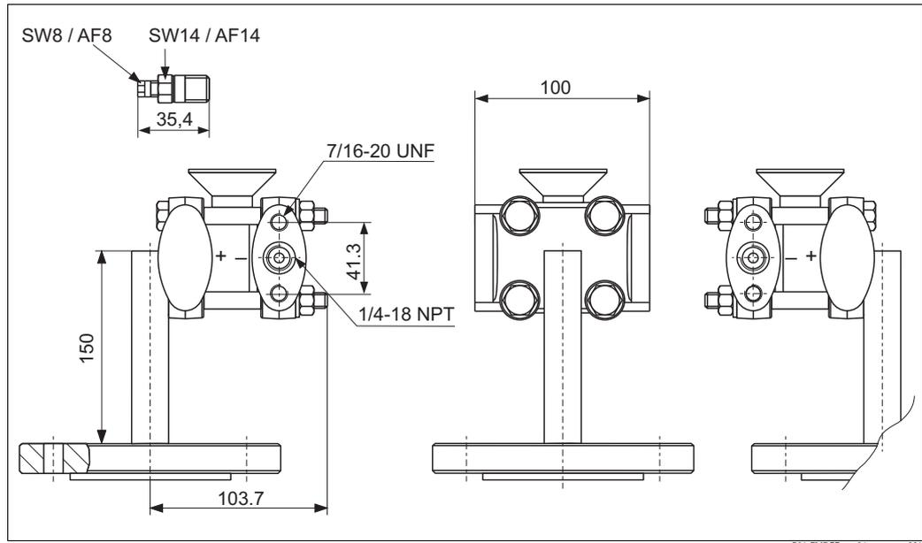
Low-pressure side: connection 1/4-18 NPT, mounting optionally 7/16-20 UNF incl. 1 vent valve AISI 316L (1.4404), Side flange material of the basic device: AISI 316L (1.4435 or 1.4404)
