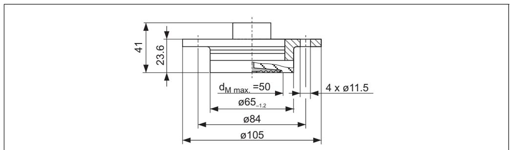
Process connection FMD78, surface roughness of the surfaces in contact with the media  $R_a \leq 0.76 \mu\text{m}$  (29.9  $\mu\text{in}$ ) as standard. Lower surface roughness on request.
