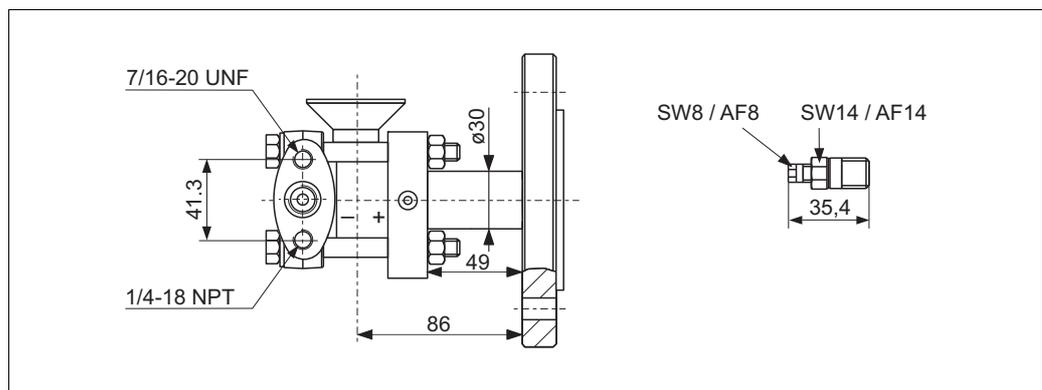
Low-pressure side: connection 1/4-18 NPT, mounting optionally 7/16-20 UNF incl. 1 vent valve AISI 316L (1.4404), Side flange material of the basic device: AISI 316L (1.4435 or 1.4404)
