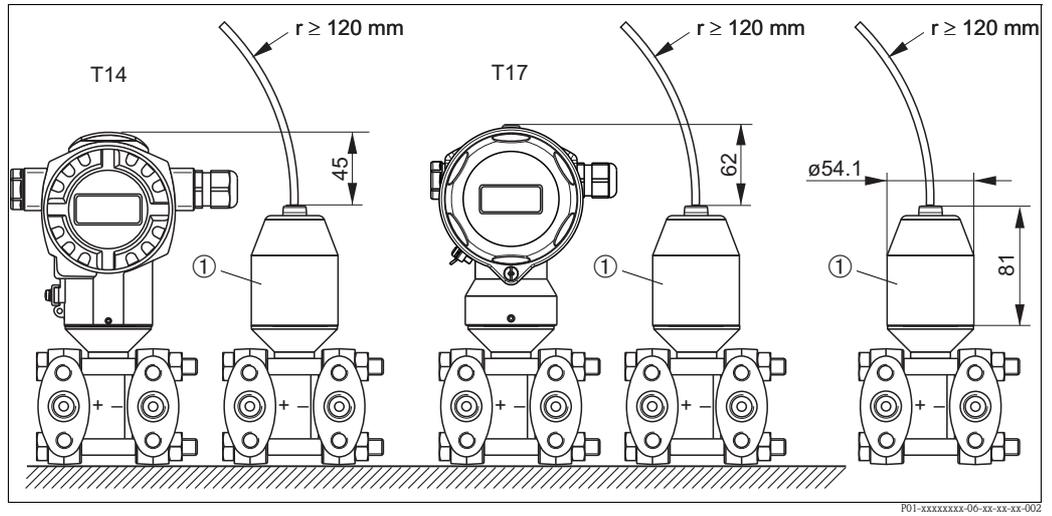
Reduction of the installation height of the process connection when using the separate housing.
