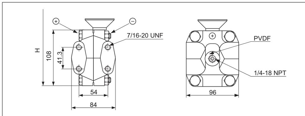
Process connection PMD70, version G, PVDF Inlay, MWP 10 bar (150 psi), OPL max. 15 bar (225 psi), process temperature  $T = -10$  to  $+60^{\circ}\text{C}$  (14 to  $+140^{\circ}\text{F}$ )
