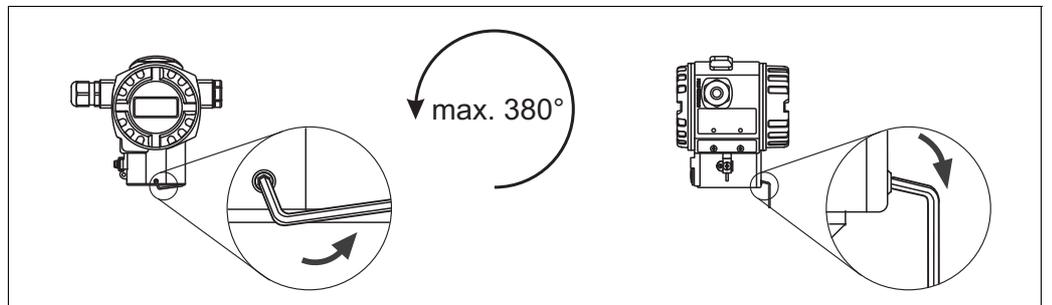
Aligning the housing by releasing the setscrew
