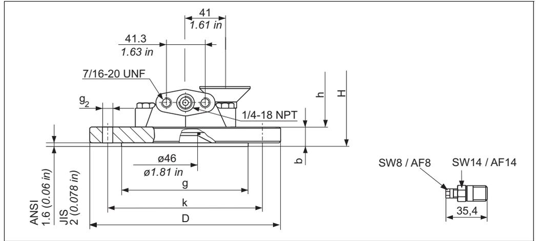
Process connection FMD76, high-pressure side: ANSI or JIS flange, Low-pressure side: connection 1/4-18 NPT
