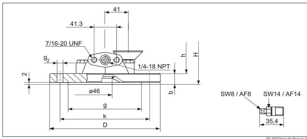
Process connection FMD76, high-pressure side: EN/DIN flange, Low-pressure side: connection 1/4-18 NPT
