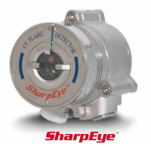
The new 40/40 UV Flame Detector detects hydrocarbon-based fuel and gas fires, invisible hydrogen flames, and fires from hydrides, ammonia, silane and other organics. The 40/40U-UB is the most durable and weather resistant UV flame detector currently on the market. Its new features include a heated window, to eliminate condensation and icing; HART capabilities, for digital communications; lower power requirements; and a compact, lighter design.
