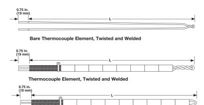
Thermocouple Element, Butt Welded
