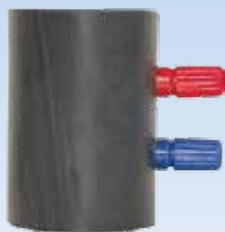
CT-55 CONDUCTIVITY CUP FOR E-COAT PAINT PROCESS
