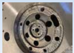
Pictured is a die that a customer sent us. The die was worn and needed it to be built back up for re-machining.
